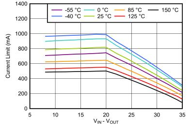
Figure 6-1. Current-Limit vs V<sub>Head-room</sub> Behavior (New Chip)
