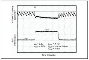
**FIGURE 2-23:** Load Transient.
