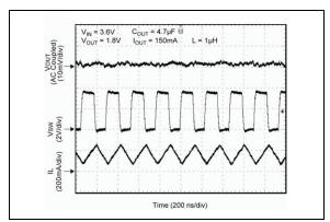
FIGURE 2-18: Switching Waveform - Continuous Mode.
