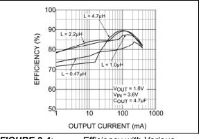
**FIGURE 2-4:** Efficiency with Various Inductors.
