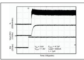
**FIGURE 2-21:** Start-Up Waveform.
