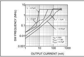
FIGURE 5-2: Switching Frequency vs. Inductance.
