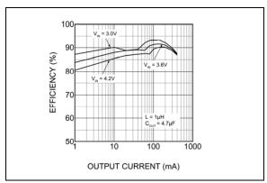
FIGURE 5-1: Efficiency under Load.
