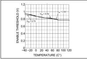
FIGURE 2-13: Enable Threshold vs. Temperature.
