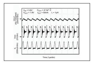
**FIGURE 2-17:** Switching Waveform - Discontinuous Mode.
