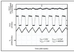
**FIGURE 2-20:** Switching Waveform -Continuous Mode.
