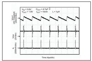
**FIGURE 2-16:** Switching Waveform - Discontinuous Mode.
