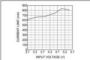
FIGURE 2-14: Current-Limit vs. Input Voltage.
