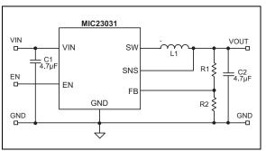
FIGURE 4-1: MIC23031-AYMT Schematic.
