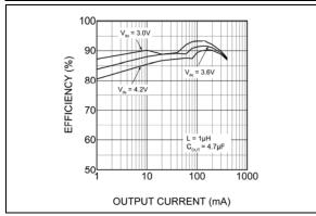
**FIGURE 2-1:** Efficiency  $(V_{OUT} = 2.5V)$ .
