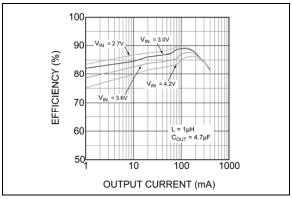
**FIGURE 2-2:** Efficiency  $(V_{OUT} = 1.8V)$ .
