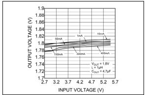
**FIGURE 2-6:** Output Voltage vs. Input Voltage.
