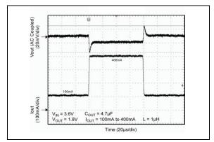
FIGURE 2-26: Load Transient.
