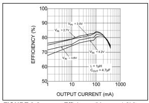
**FIGURE 2-3:** Efficiency  $(V_{OUT} = 1.2V)$
