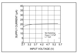
FIGURE 2-5: Quiescent Current vs. Input Voltage.
