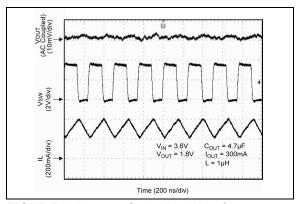
**FIGURE 2-19:** Switching Waveform -Continuous Mode.
