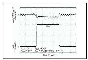
FIGURE 2-25: Load Transient.
