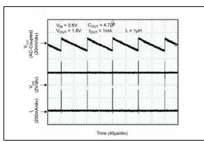
**FIGURE 2-15:** Switching Waveform - Discontinuous Mode.
