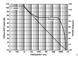
Figure 22. Open-Loop Gain and Phase vs. Frequency
