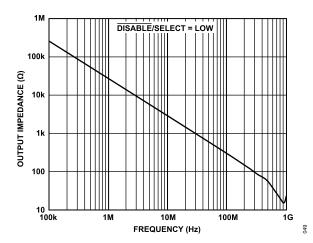
Figure 54. Output Disabled—Impedance vs. Frequency
