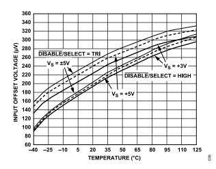
Figure 43. Input Offset Voltage vs. Temperature
