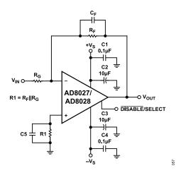
Figure 63. Wideband Inverting Gain Configuration
