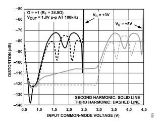
Figure 30. Harmonic Distortion vs. Input Common-Mode Voltage, DISABLE/ SELECT = Trisate or Open
