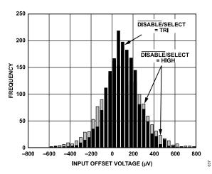
Figure 42. Input Offset Voltage Distribution
