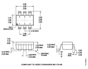
Figure 70. 6-Lead Small Outline Transistor Package [SOT-23] (RJ-6) Dimensions shown in millimeters
