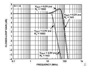
Figure 18. Small Signal Frequency Response for Various R<sub>LOAD</sub> Values
