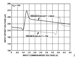
Figure 45. Input Offset Voltage vs. Input Common-Mode Voltage, V<sub>S</sub> = 5 V
