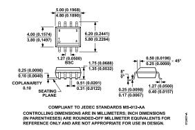
Figure 69. 8-Lead Standard Small Outline Package [SOIC\_N]
