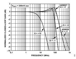
Figure 8. Small Signal Frequency Response for Various Gains
