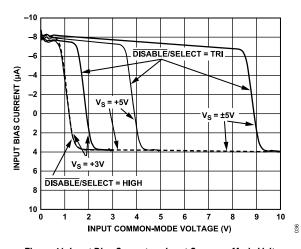
Figure 41. Input Bias Current vs. Input Common-Mode Voltage
