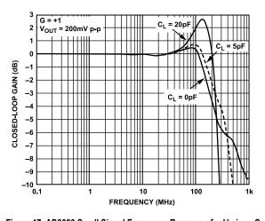
Figure 17. AD8028 Small Signal Frequency Response for Various C<sub>LOAD</sub> Values
