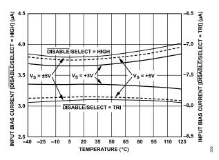
Figure 40. Input Bias Current vs. Temperature
