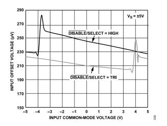
Figure 44. Input Offset Voltage vs. Input Common-Mode Voltage,  $V_S = \pm 5 \text{ V}$
