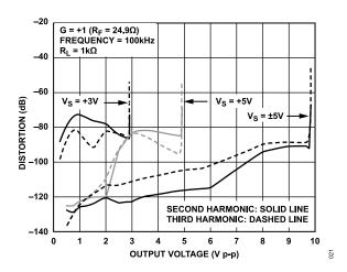
Figure 26. Harmonic Distortion vs. Output Voltage
