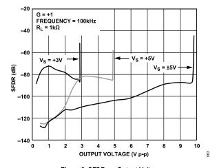
Figure 2. SFDR vs. Output Voltage
