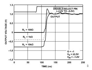
Figure 56. Enable Turn On Timing
