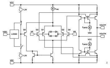
Figure 60. Simplified Input Stage
