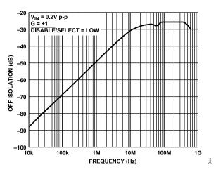
Figure 49. Off Isolation vs. Frequency
