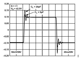
Figure 35. Small Signal Transient Response with Capacitive Load
