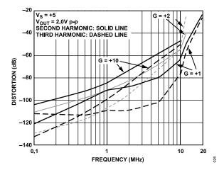
Figure 31. Harmonic Distortion vs. Frequency and Gain
