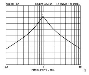
Figure 68. Band-Pass Filter Response
