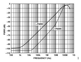
Figure 48. Power Supply Rejection Ratio (PSRR) vs. Frequency
