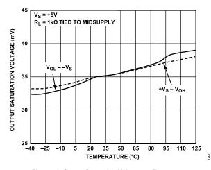
Figure 52. Output Saturation Voltage vs. Temperature
