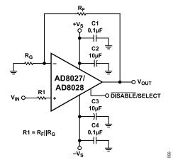
Figure 62. Wideband Noninverting Gain Configuration
