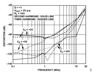
Figure 25. Harmonic Distortion vs. Frequency and Supply Voltage
