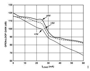
Figure 53. Open-Loop Gain vs. Load Current
