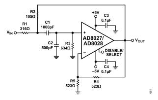
Figure 67. Band-Pass Filter Schematic
