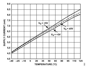
Figure 58. Quiescent Supply Current vs. Temperature and Supply Voltage
