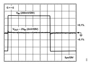
Figure 38. Long-Term Settling Time
