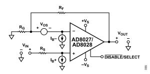
Figure 61. Op Amp DC Error Sources
