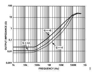
Figure 51. Output Enabled—Impedance vs. Frequency
