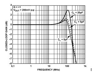
Figure 14. AD8027 Small Signal Frequency Response for Various C<sub>LOAD</sub> Values
