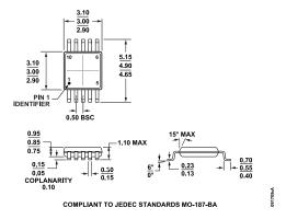
Figure 71. 10-Lead Mini Small Outline Package [MSOP]
