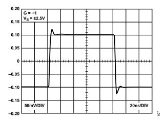
Figure 32. Small Signal Transient Response
