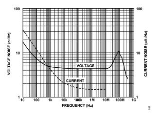
Figure 23. Voltage and Current Noise vs. Frequency
