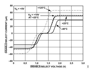
Figure 55. DISABLE/SELECT Current vs. DISABLE/SELECT Voltage and Temperature
