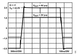
Figure 33. Large Signal Transient Response, G = +1
