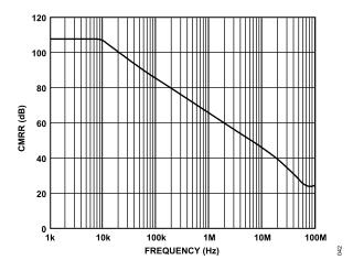
Figure 47. Common-Mode Rejection Ratio (CMRR) vs. Frequency
