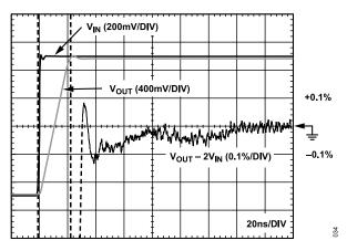
Figure 39. 0.1% Short-Term Settling Time
