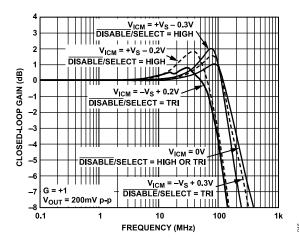
Figure 20. Small Signal Frequency Response vs. Frequency for Various Input Common-Mode Voltages
