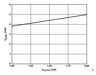
Figure 81. I<sub>AVDD</sub> vs. I<sub>OUTFS</sub> at AVDD = 1.8 V
