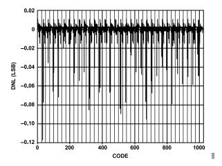
Figure 61. AD9705 Typical Uncalibrated DNL
