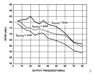
Figure 12. SFDR vs. f<sub>OUT</sub> and I<sub>OUTFS</sub> at 175 MSPS
