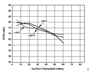
Figure 23. SFDR vs.  $f_{OUT}$  and Temperature at 175 MSPS
