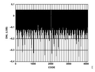
Figure 63. AD9706 Typical Uncalibrated DNL
