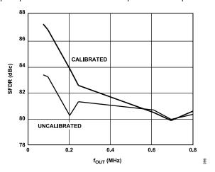
Figure 86. AD9707 SFDR vs.  $f_{OUT}$  at 175 MSPS and  $I_{OUTFS}$  = 2 mA
