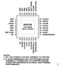
Figure 4. AD9706 Pin Configuration
