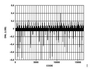
Figure 20. Typical Uncalibrated DNL
