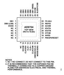
Figure 6. AD9704 Pin Configuration
