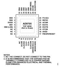
Figure 5. AD9705 Pin Configuration
