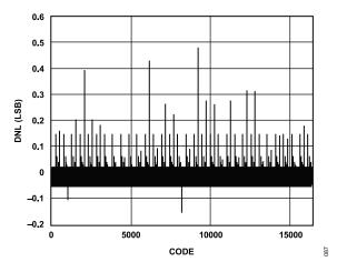
Figure 22. Typical Calibrated DNL
