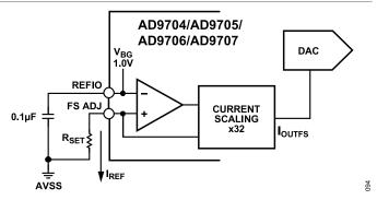
Figure 77. Internal Reference Configuration
