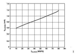
Figure 85. I<sub>CLKVDD</sub> vs. f<sub>CLOCK</sub> (Differential Clock Mode) at CLKVDD = 1.8 V
