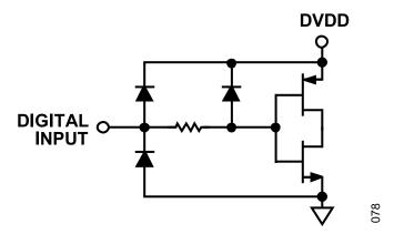
Figure 79. Equivalent Digital Input
