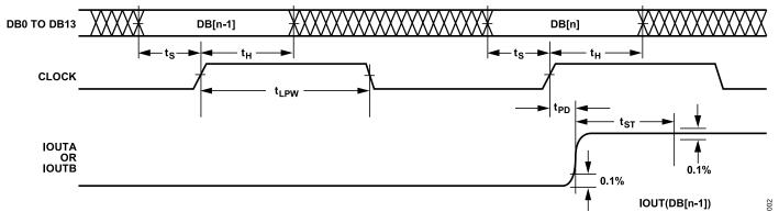
Figure 2. Parallel Data Interface Timing Diagram
