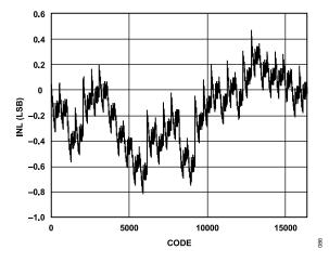
Figure 21. Typical Calibrated INL
