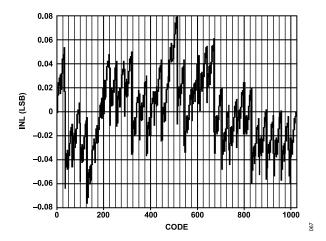
Figure 60. AD9705 Typical Uncalibrated INL
