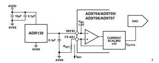
Figure 78. External Reference Configuration
