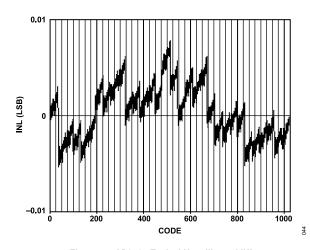
Figure 47. AD9705 Typical Uncalibrated INL
