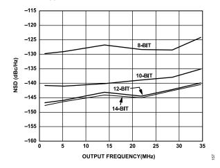
Figure 57. AD9704/AD9705/AD9706/AD9707 NSD vs. f<sub>OUT</sub> at 0 dBFS, 80 MSPS
