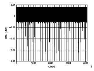
Figure 50. AD9706 Typical Uncalibrated DNL
