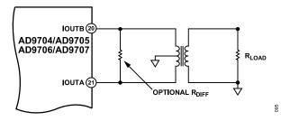
Figure 88. Differential Output Using a Transformer
