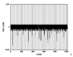
Figure 48. AD9705 Typical Uncalibrated DNL
