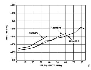
Figure 15. NSD vs. f<sub>OUT</sub> and f<sub>CLOCK</sub> at 0 dBFS
