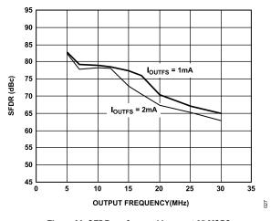
Figure 30. SFDR vs. f<sub>OUT</sub> and l<sub>OUTFS</sub> at 65 MSPS
