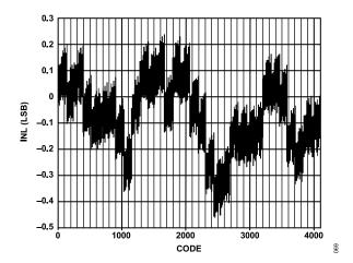
Figure 62. AD9706 Typical Uncalibrated INL
