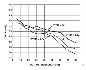
Figure 13. SFDR vs.  $f_{OUT}$  and OTCM at 175 MSPS
