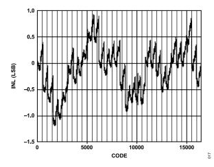
Figure 19. Typical Uncalibrated INL
