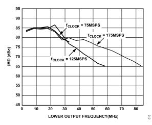
Figure 17. Dual-Tone IMD vs. Lower  $f_{\rm OUT}$  and  $f_{\rm CLOCK}$  at 0 dBFS
