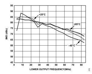
Figure 18. Dual-Tone IMD vs. Lower f<sub>OUT</sub> and Temperature at 0 dBFS, 175
