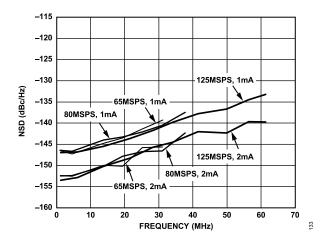
Figure 33. NSD vs.  $f_{\text{OUT}}$ ,  $f_{\text{CLOCK}}$ , and  $I_{\text{OUTFS}}$  at 0 dBFS
