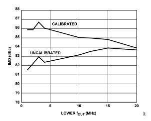
Figure 87. IMD vs. Lower  $f_{OUT}$  at 175 MSPS and  $I_{OUTFS}$  = 2 mA
