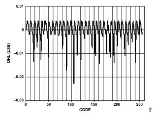
Figure 59. AD9704 Typical Uncalibrated DNL
