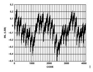
Figure 49. AD9706 Typical Uncalibrated INL
