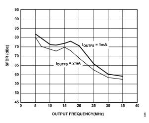
Figure 31. SFDR vs.  $f_{OUT}$  and  $I_{OUTFS}$  at 80 MSPS
