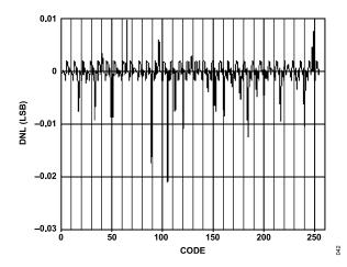
Figure 46. AD9704 Typical Uncalibrated DNL
