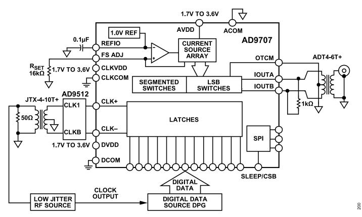
Figure 70. Basic AC Characterization Test Setup
