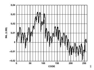
Figure 58. AD9704 Typical Uncalibrated INL
