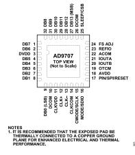
Figure 3. AD9707 Pin Configuration
