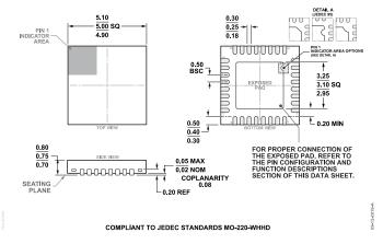
Figure 91. 32-Lead Lead Frame Chip Scale Package [LFCSP] 5 mm × 5 mm Body and 0.75 mm Package Height (CP-32-7) Dimensions shown in millimeters
