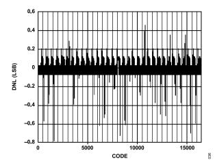
Figure 39. Typical Uncalibrated DNL
