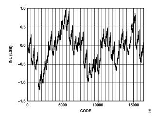
Figure 38. Typical Uncalibrated INL
