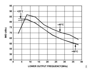
Figure 37. Dual-Tone IMD vs. Lower  $f_{OUT}$  and Temperature at 80 MSPS,  $I_{OUTFS}$  = 2 mA and 0 dBFS
