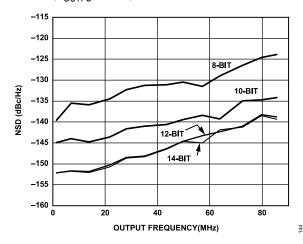
Figure 44. AD9704/AD9705/AD9706/AD9707 NSD vs.  $f_{\rm OUT}$  at 0 dBFS, 175 MSPS
