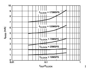
Figure 82. I<sub>DVDD</sub> vs. f<sub>OUT</sub>/f<sub>CLOCK</sub> Ratio at DVDD = 3.3 V
