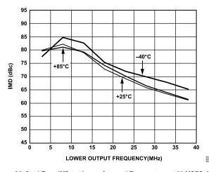
Figure 36. Dual-Tone IMD vs. Lower  $f_{OUT}$  and Temperature at 80 MSPS,  $I_{OUTFS}$  = 1 mA and 0 dBFS
