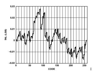
Figure 45. AD9704 Typical Uncalibrated INL
