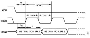
Figure 75. Timing Diagram for SPI Register Write
