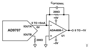
Figure 89. Unipolar Buffered Voltage
