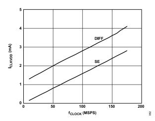
Figure 84. I<sub>CLKVDD</sub> vs. f<sub>CLOCK</sub> at CLKVDD = 3.3 V
