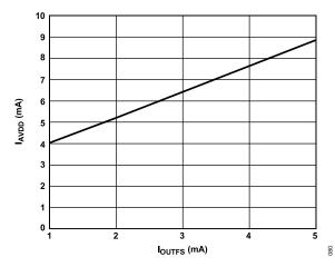
Figure 80. I<sub>AVDD</sub> vs. I<sub>OUTFS</sub> at AVDD = 3.3 V
