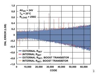
Figure 8. Differential Nonlinearity Error vs. Code
