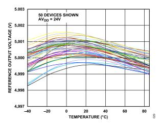
Figure 32. Reference Output Voltage vs. Temperature
