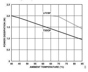
Figure 53. Maximum Power Dissipation vs. Ambient Temperature
