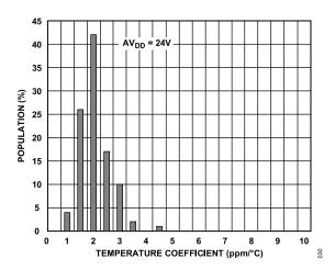
Figure 33. Reference Temperature Coefficient Histogram
