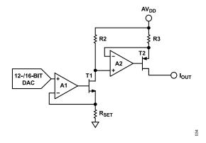
Figure 38. Voltage-to-Current Conversion Circuitry
