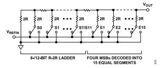
Figure 37. DAC Ladder Structure
