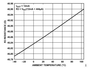
Figure 49. R3 Resistor Value vs. Temperature
