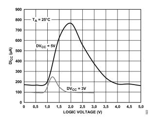
Figure 25. DI<sub>CC</sub> vs. Logic Input Voltage
