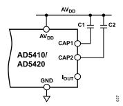
Figure 44. I<sub>OUT</sub> Filtering Capacitors
