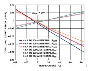
Figure 13. Total Unadjusted Error vs. Temperature
