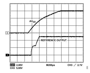
Figure 28. Reference Turn-on Transient
