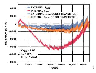
Figure 7. Integral Nonlinearity Error vs. Code
