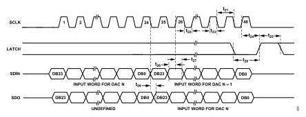
Figure 4. Daisy-Chain Mode Timing Diagram
