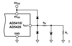
Figure 51. Output Transient Voltage Protection
