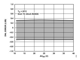
Figure 19. Differential Nonlinearity Error vs. AV<sub>DD</sub>, Internal R<sub>SET</sub>
