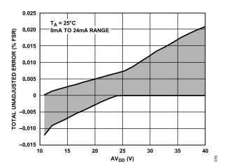
Figure 20. Total Unadjusted Error vs. AV<sub>DD</sub>, External R<sub>SET</sub>
