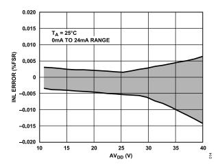
Figure 17. Integral Nonlinearity Error vs. AV<sub>DD</sub>, Internal R<sub>SET</sub>
