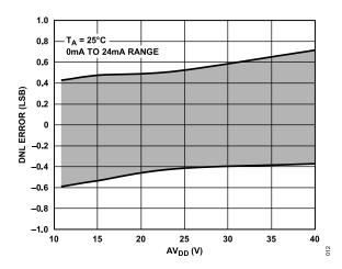
Figure 18. Differential Nonlinearity Error vs.  $AV_{DD}$ , External  $R_{SET}$
