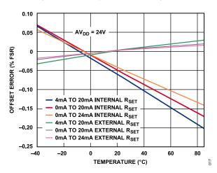
Figure 14. Offset Error vs. Temperature
