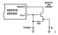
Figure 41. External Boost Configuration
