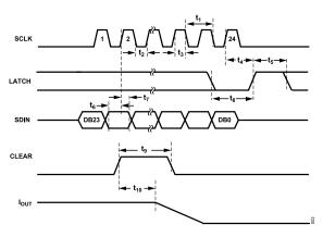
Figure 2. Write Mode Timing Diagram
