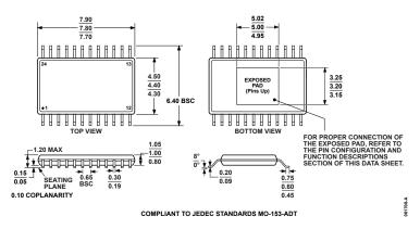
Figure 56. 24-Lead Thin Shrink Small Outline Package, Exposed Pad [TSSOP\_EP]
