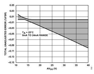
Figure 21. Total Unadjusted Error vs. AV<sub>DD</sub>, Internal R<sub>SET</sub>
