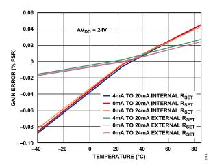
Figure 15. Gain Error vs. Temperature
