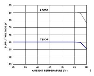
Figure 54. Maximum Supply Voltage vs. Ambient Temperature
