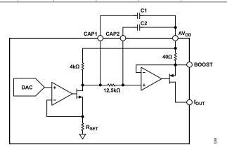
Figure 45. IOUT Filter Circuitry
