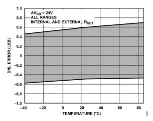
Figure 12. Differential Nonlinearity Error vs. Temperature
