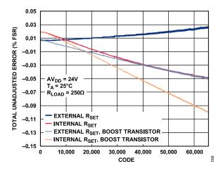
Figure 9. Total Unadjusted Error vs. Code
