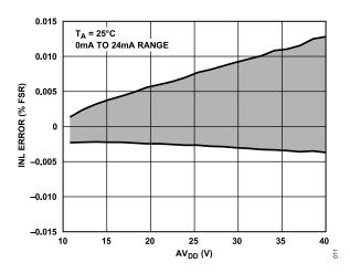
Figure 16. Integral Nonlinearity Error vs. AV<sub>DD</sub>, External R<sub>SET</sub>
