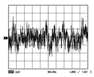
Figure 29. Reference Noise (0.1 Hz to 10 Hz Bandwidth)
