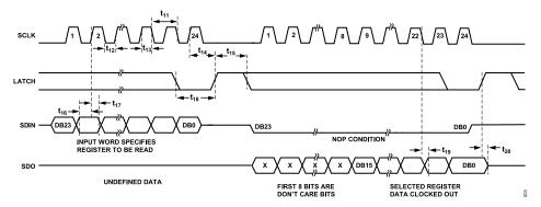
Figure 3. Readback Mode Timing Diagram
