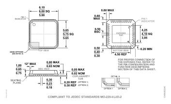
Figure 57. 40-Lead Lead Frame Chip Scale Package [LFCSP]
