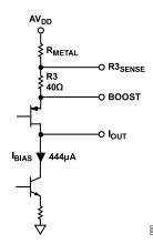
Figure 48. Structure of Current Output Circuit
