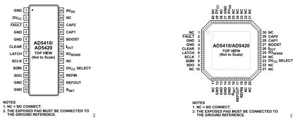
Figure 5. TSSOP Pin Configuration
