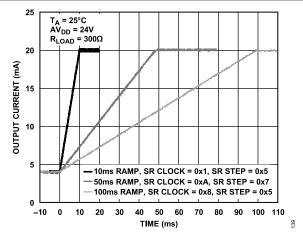
Figure 43. Output Current Slewing Under Control of the Digital Slew Rate
