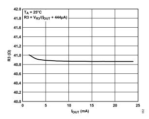
Figure 50. R3 Resistor Value vs. IOUT
