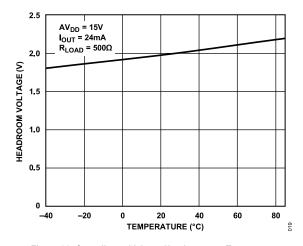
Figure 22. Compliance Voltage Headroom vs. Temperature
