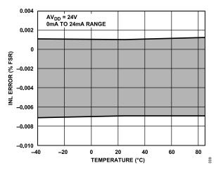
Figure 10. Integral Nonlinearity Error vs. Temperature, Internal R<sub>SET</sub>
