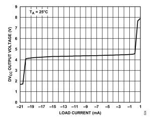
Figure 27. DV<sub>CC</sub> Output Voltage vs. Load Current
