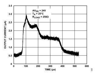
Figure 23. Output Current vs. Time on Power-Up
