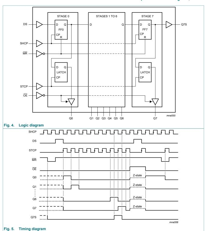
8-bit serial-in/serial-out or parallel-out shift register; 3-state
